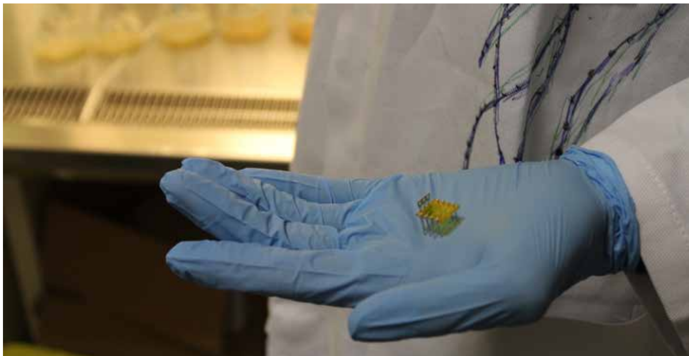
Organic light-emitting diode on glass substrate to test suitable materials for medical applications.
