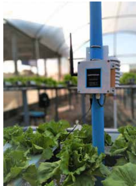
Camnexus-IoT sensors network: Meteo-Plus© sensor for integrated weather station and water quality real-time monitoring. First network installed in hydroponic greenhouse farm in Brazil.
